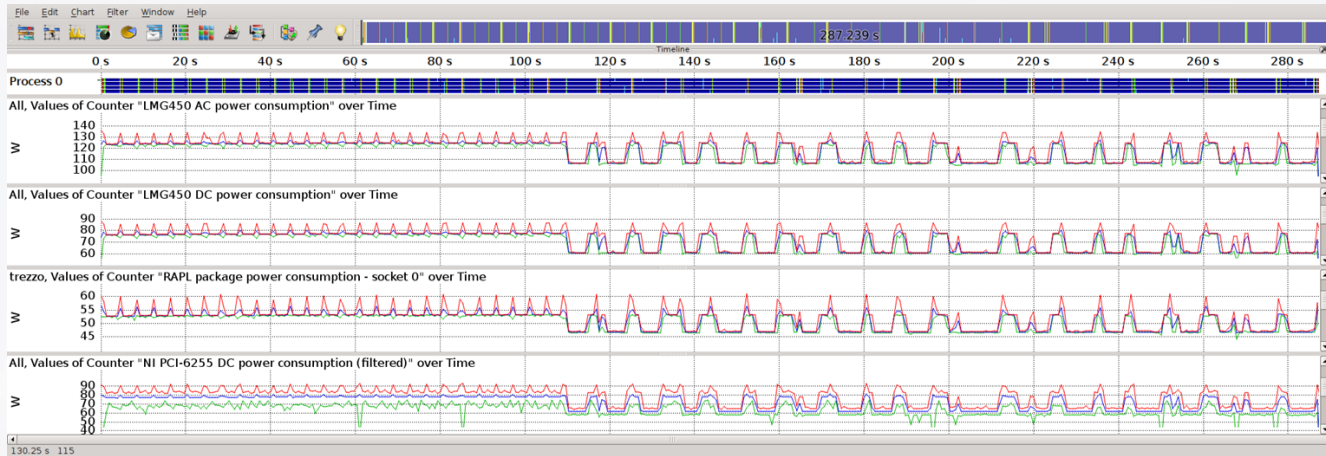
SPEC OMP applu, measurements with ZES-ZIMMER LMG 450/dataheap, RAPL, and HAEC infrastructure [HIS+13]
